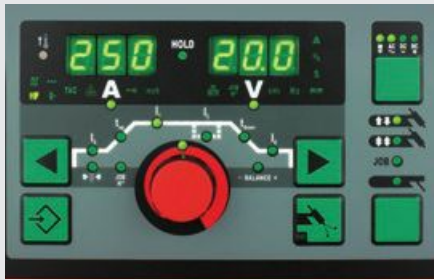
/ Control panel of MW 2500 Job
